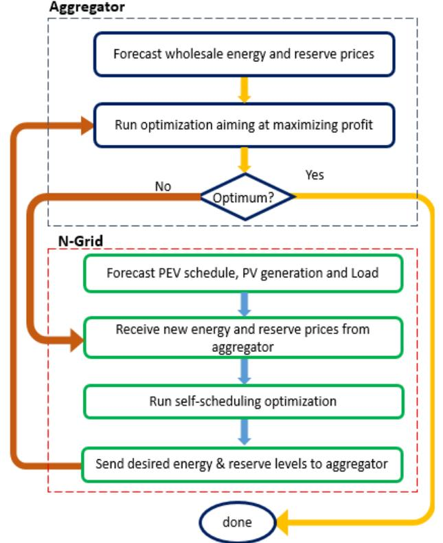
Figure 1. The flowchart of aggregator and n-Grids' interaction.
