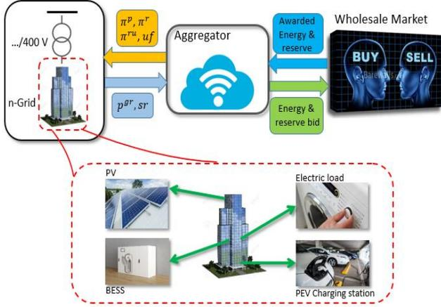
Figure 2. A typical nano-Grid and its interaction with the aggregator.
