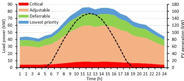
Figure 3. The n-Grid's different load type and PV power data.
