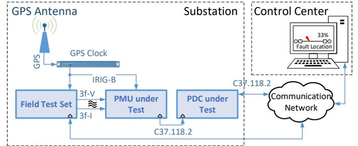
Figure 7: Application Test Setup.
