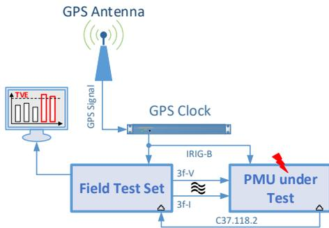
Figure 5: PMU Test Setup with Intrusion.
