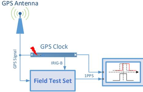
Figure 4: Time Module Test Setup Showing an Intrusion.
