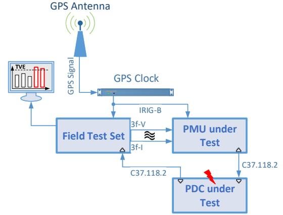
Figure 6: PDC Test Setup with Intrusion.
