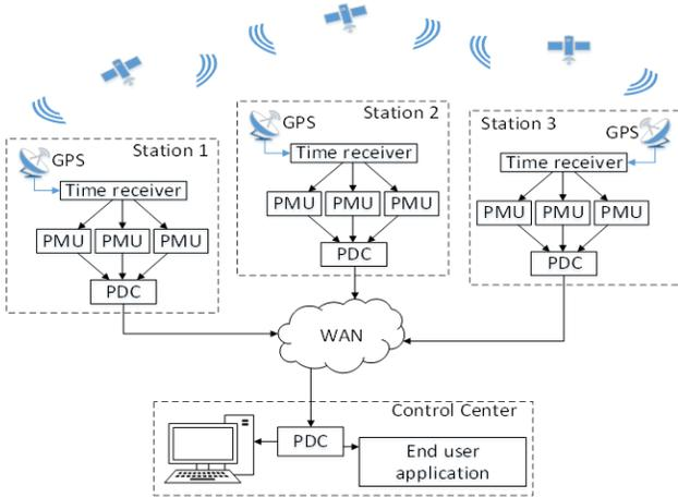
Figure 1: Example of Synchrophasor System Components.
